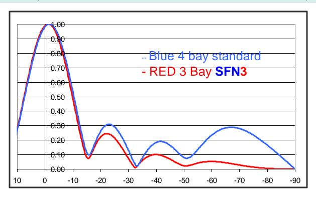
The above plot is a comparison of a 3-bay SFN3 to a 4-bay standard slot antenna. The SFN3 has 14 dB less RFR hitting the ground. These small, but powerful antennas are perfect for distributed ATSC 3.0 transmission. They will let you place these antennas nearly anywhere you can think of.. Call us for more information.
